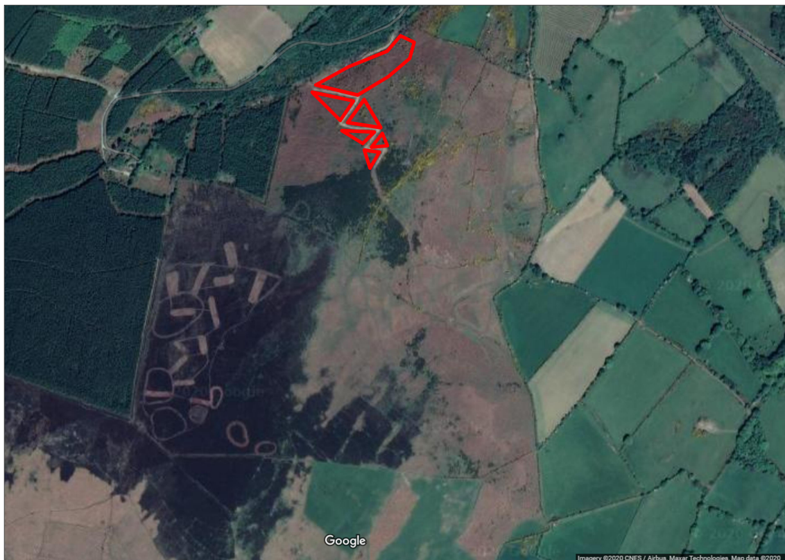
Figure 4. Additional tree planting measures are recommended at the locations indicated along the track created in 2020 (Google maps) to further stabilise the slopes here.
